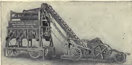
Champion Steel Rock Crusher. Mounted with Elevator, Screen and Portable Stone Bin. Made in several sizes, 15 to 300 tons daily.
